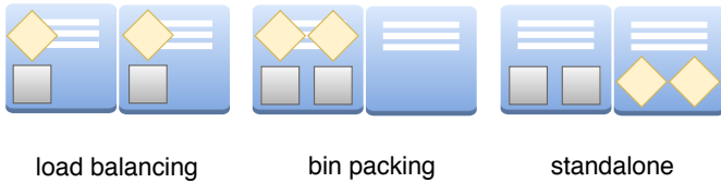
Fig. 3: Placement under different schemes (diamonds represent PS and worker in job 1; squares represent those of job 2)
