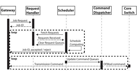
Fig. 4. The control logic between the controller and a gateway server.
