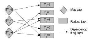
Fig. 2. An illustration of the MapReduce job model.
