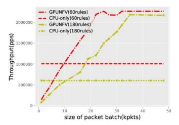
Figure 2: Throughput: GPUNFV vs. CPU-only processing
