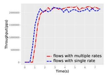
Figure 3: Throughput of GPUNFV with multiple flow rates
