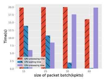
Figure 4: Time used by CPU and GPU threads
