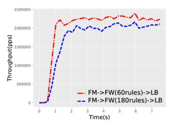
Figure 6: Throughput with dynamic batch sizing
