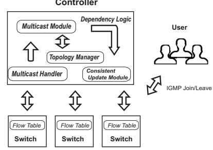
Fig. 6: Main Components in the Prototype System
