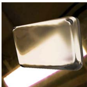
Fig. 2. Blurring effects of background details showing through a wedge-shaped object. The right side is thicker than the left . The image of the lamp is blurred more at the right
